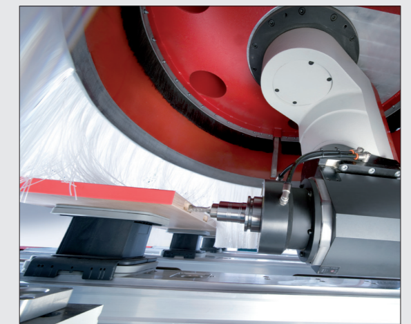
Robot head with endlessly rotating A- and C-axes
