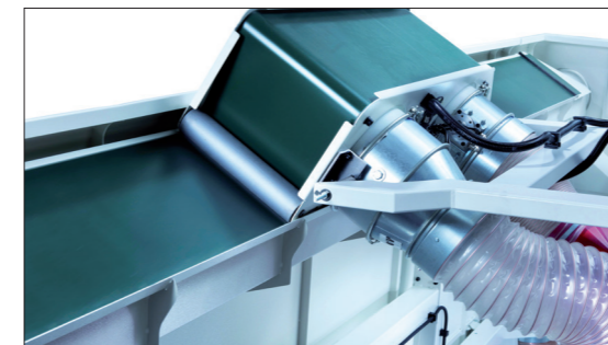
Integrated extraction concept for reduced height (optional)
