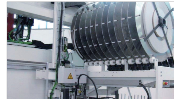
12-fold edge magazine, servo-controlled
